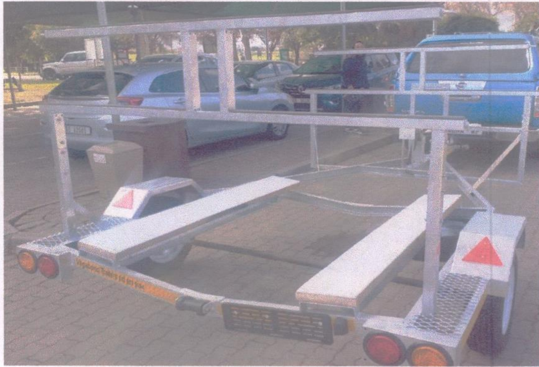
Trailer to transport Rubber Duck and 4x Kayaks manufactured for Mossel Bay Municipality
